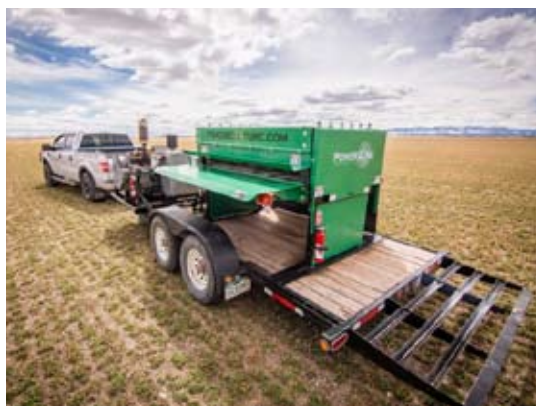
The Fiber Track™ decorticator can process up to 10 tons/hr.
