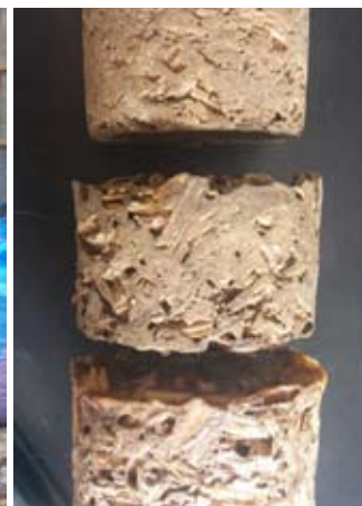
Processing hemp fiber at Adrar Nough; right, new hemp-clay composites developed by Monika Brümmer
