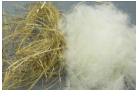
Hemp fiber, before and after cottonization
