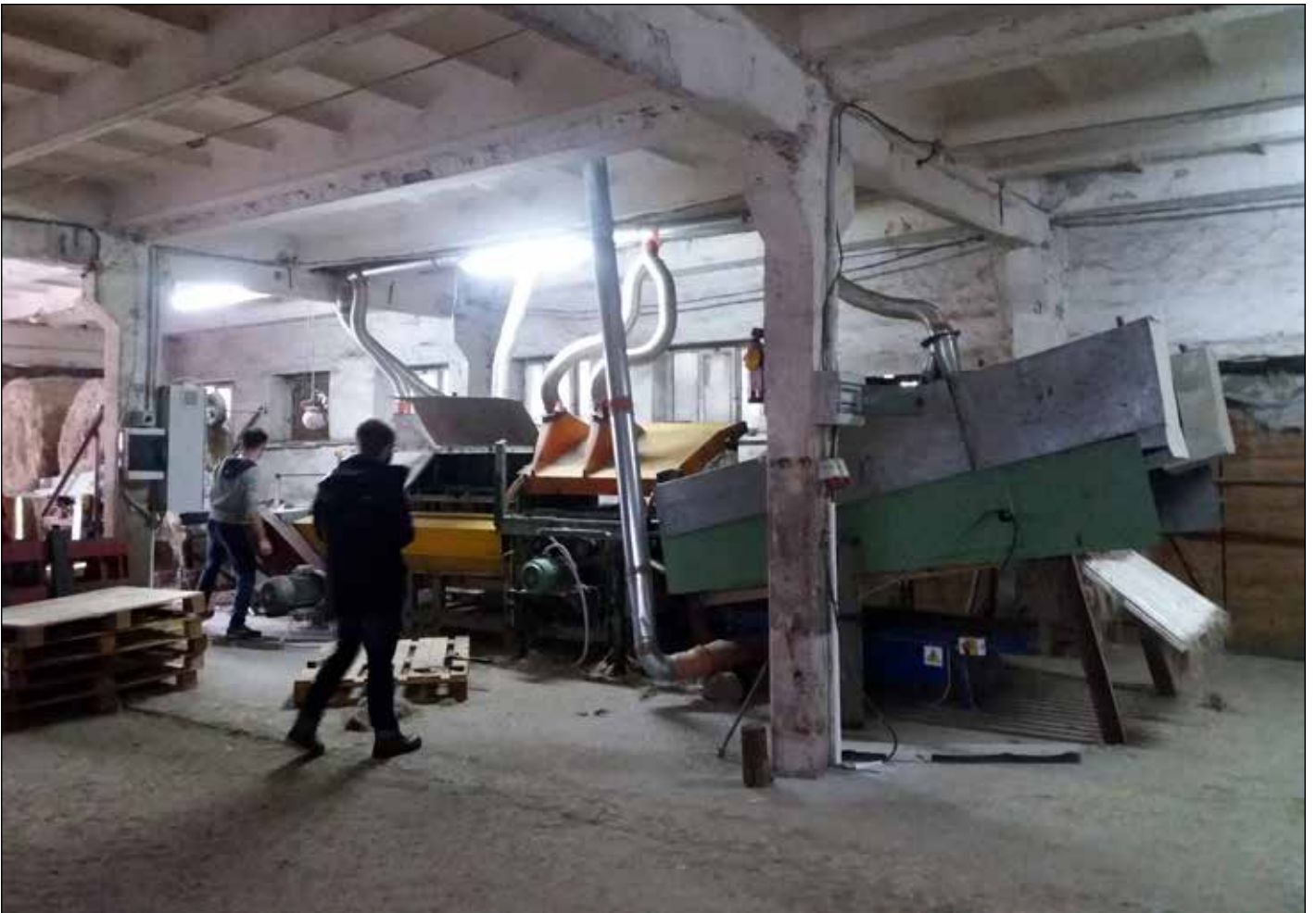
A re-engineered decorticating line used to produce hurd for hempcrete and insulation materials.
